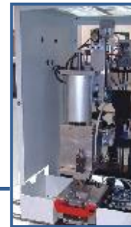
Dosing gun with pressure and volume control.
